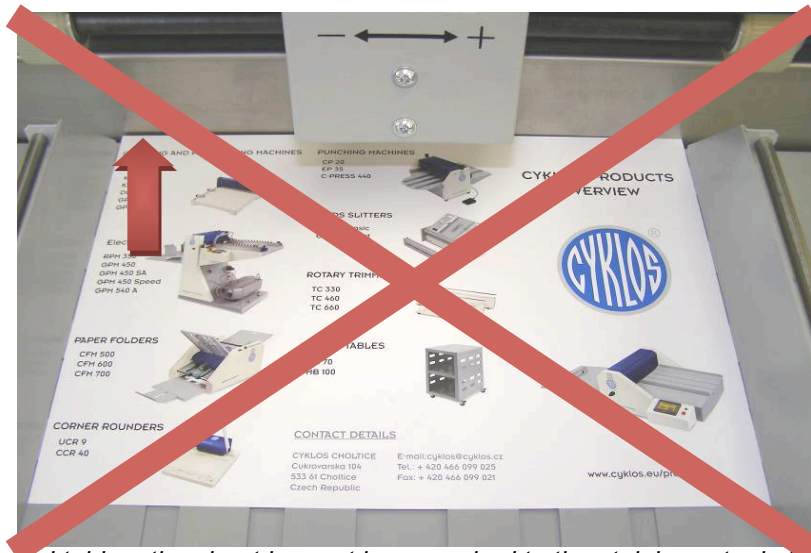
Fig. 10: Incorrectly prepared table – the sheet has not been pushed to the stainless steel plate along its whole length
