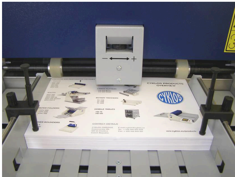
Fig. 15: Example of correct placement of paper pile
