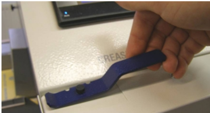
Fig. 17: Pulling callipers to the upper position
