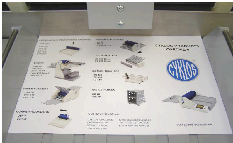
Fig. 9: Correctly prepared table – the sheet has been pushed to the stainless steel plate
