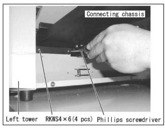
5. Install the connecting chassis at the right tower.
