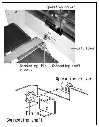
(2) Using Phillips screwdriver, fix the connecting chassis with RKWS4x4 screws (4 locations).
