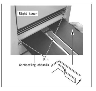
6. Fit the bridge side plate to the connecting chassis with RKWS4x6 screws (2 pcs).
