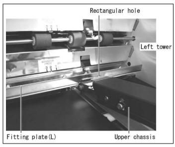
(2) Insert the right side tip of the upper chassis in the square hole on the bridge side plate, and fit the upper chassis to the connecting chassis using the upper chassis fitting knob.
