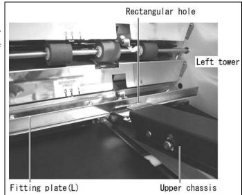
(2) Insert the right side tip of the upper chassis in the sqaure hole on the bridge side plate, and fit the upper chassis to the connecting chassis using the upper chassis fitting knob.
