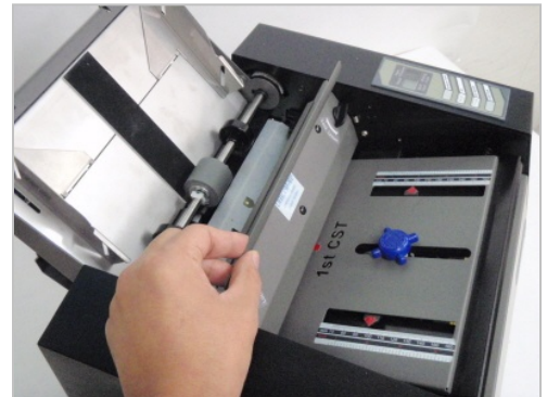
[Open the cover and remove the jam]
