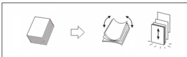
[Pressure seal form handling before using]
