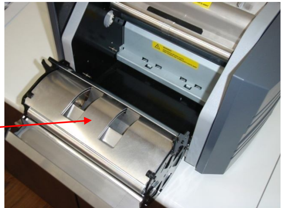
Folding Drum in the partially open position
