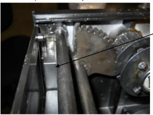
8. Now you will adjust the second motor position plate so that the gap is also located in between the U shape of the sensor. Then you may tighten the bolts.
