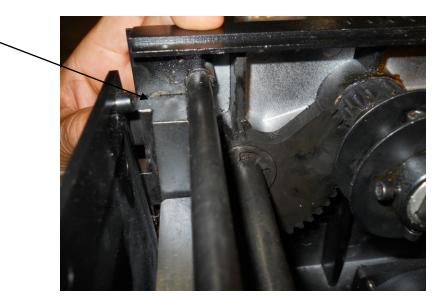
4. Now you will turn the first motor position plate so that the gap that is on it, is located in between the sensor's U shape
