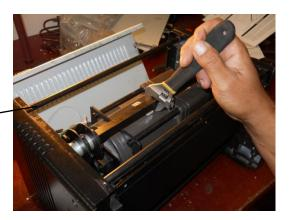
3. Once all the bolts are loosened on the first plate, you will have to turn the shaft with the tool so that the gear (connect block- p# A20701) is in the up position.
