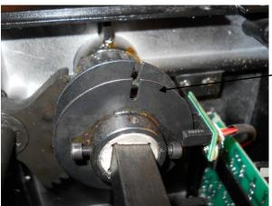
7. Once all the bolts are loose, you will need to turn the shaft so that the gear (left connect block-P# AS20701) is in the down position.
