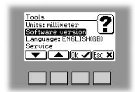
Select Software version with the [arrow] button and press the [OK] button. This screen, and sub screens show the software version for the different modules in the booklet making system.
