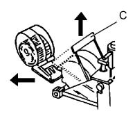
The staple cartridges, containing approximately 5000 staples per cartridge. Cartridge may be removed either for renewal or for jam clearance.
