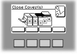
When the message "Close Cover(s)" is displayed any of the interlock switches are actuated.
