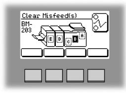
In general, fault codes indicate a misfeed condition. When a misfeed occurs, the message "Clear Misfeed(s)", a code and the jam area will be displayed. See section 5. Clearing Misfeeds, for how to clear a misfeed.
