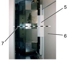
By loosening the knob (4), the docking assembly can be individually positioned for custom paper sizes.
