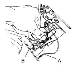
**5** Lift out the head, allowing it to rotate around the front end. The stapler assembly is spring loaded and will follow the rotation of the stapler.
