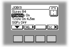
Select the option you want to change with the [arrow] button and then press the [Change] button. See section 2. Making Booklets for how to set up each separate option.
