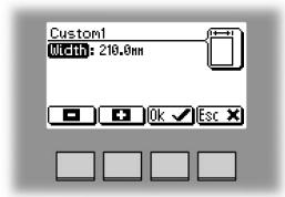
The paper size can now be changed in increments of 0.1 mm or approx. 0.01 inches. Press the [OK] button to confirm.
