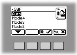
Select [Auto], [Mode 1], [Mode 2], [Mode 3], [Mode 4] or [Off] with the [arrow] button and press the [OK] button.
