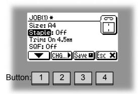
Example 4: In this screen pressing button 3 will save the current settings for job No 1. The asterisk on the first row shows that the settings for Job (1) has been changed, but not yet saved.
