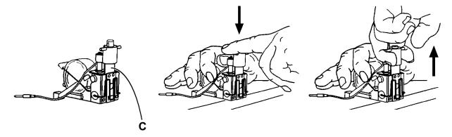
9 Remove the Stapler heads according to section 1, BASICS Check staples, Staple cartridge and Stapler head.
