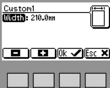
The paper size can now be changed in increments of 0.1 mm or approx. 0.01 inches. Press the [OK] button to confirm.
