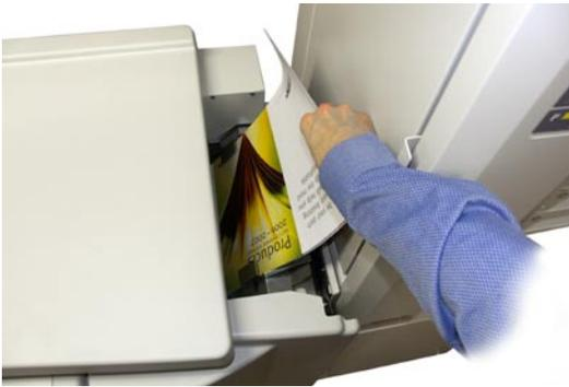
**7** Start hand feeding by inserting the sets between the side guides as illustrated.
