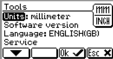
From this screen you can change units, between millimeters and inches. Select Units with the [arrow] button and press the [OK] button.
