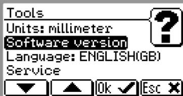
Select Software version with the [arrow] button and press the [OK] button. This screen, and sub screens show the software version for the different modules in the booklet making system.
