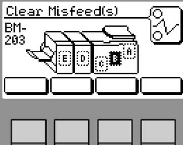
In general, fault codes indicate a misfeed condition. When a misfeed occurs, the message “Clear Misfeed(s)”, a code and the jam area will be displayed. See section 5. Clearing Misfeeds, for how to clear a misfeed.
