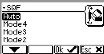
Select [Auto], [Mode 1], [Mode 2], [Mode 3], [Mode 4] or [Off] with the [arrow] button and press the [OK] button.
