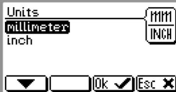
Select the millimeters or inch units and then press the [OK] button.
