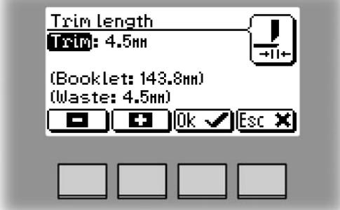
Select Trim and press the [Change] button. Select Trim length and press the [OK] button. Press the [+] or [-] buttons to fine adjust in increments of 0.5 mm or 0.02 inches. The trimmed booklet size and waste are displayed. Press the [OK] button to confirm.
