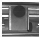
Located on the Center Spine Former. This screw enables the operator to move the Center Spine Former for different bind edge measurements. The Center Spine Former Guide should be used to determine whether the Center Spine
