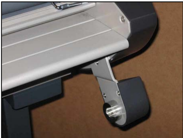
Fig. 6-7. Bottom Supply Shaft Bearing out of its Cradle
