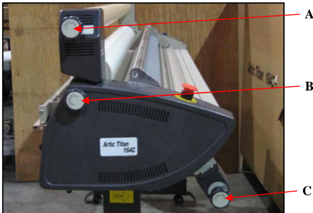
Fig. 6-21. Arctic Titan 1040 WF c Tension Adjustment Knobs and Motor
