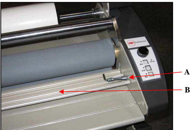
Fig. 5-9. Print Clamp and Latch
