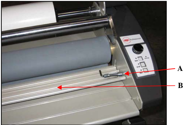
Fig. 6-4. Print Clamp and Feed Table
