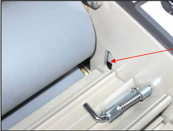
Fig. 5-2. Safety Sensor Location
