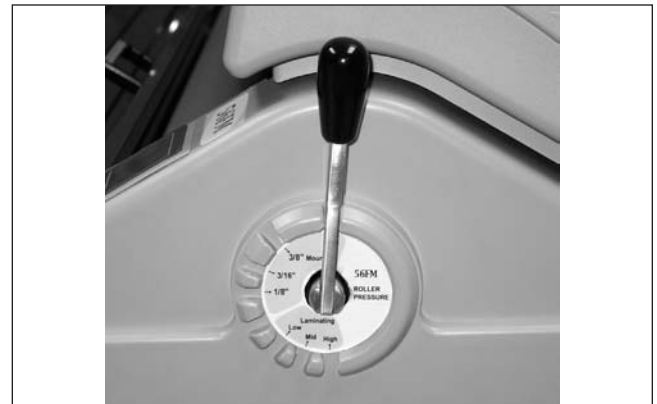
Fig. 5-3. Roller Pressure Adjustment.
