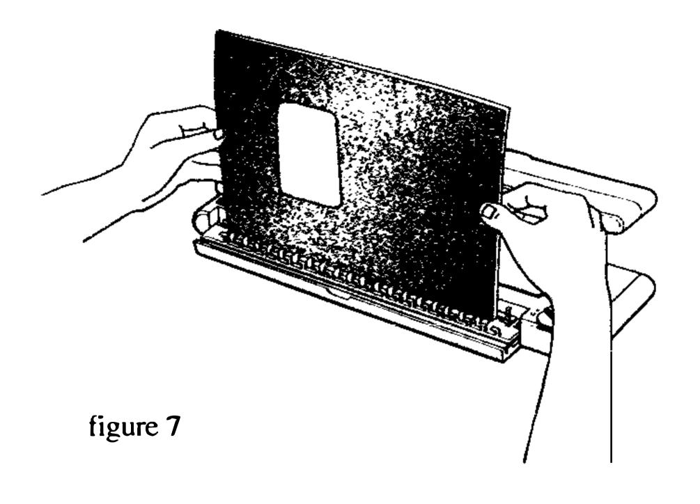
5. If you are using a cover. feed the front cover, face down, onto the comb, then the punched sheets, face down, then the back cover, face up. (figure 7).
