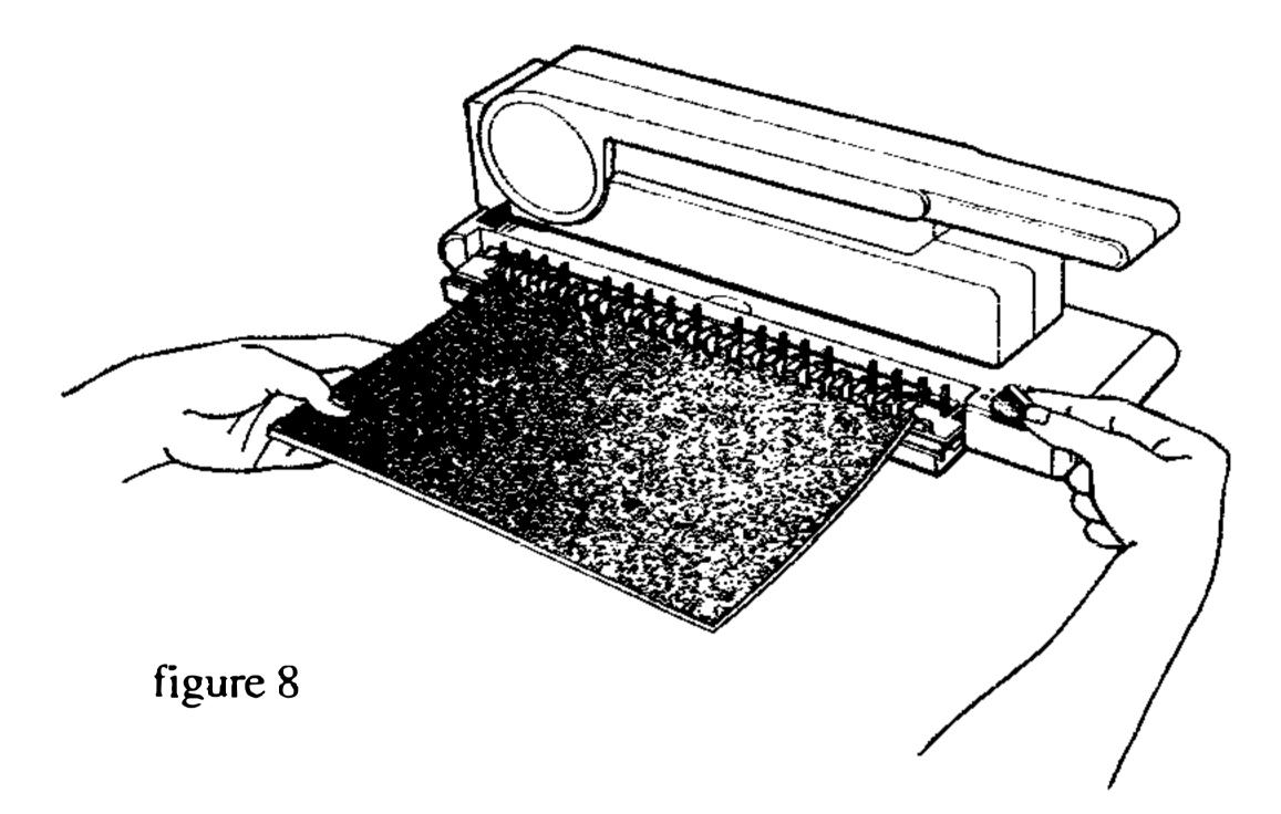
6. Close the comb by turning the binding knob counter-clockwise (figure 8).
