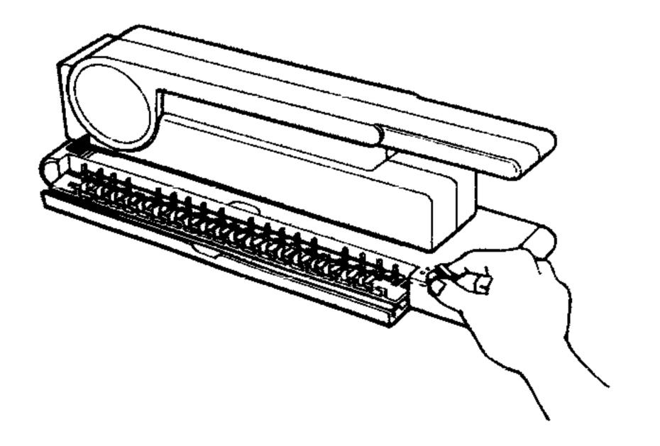
4. Open comb by turning binding knob clockwise (figure 6).
