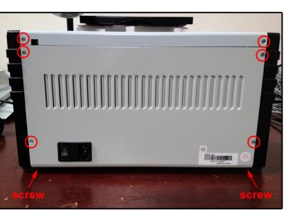
2. Remove the 8 screws on the back of the machine. Once the screws are off. you can remove the back cover from the machine.
