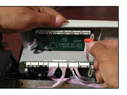
9. Disconnect each cable from old pc board and connect it to the new pc board.
