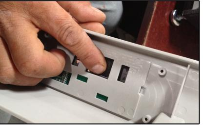
6. Push the plastic LCD cover out from the inside to remove it from the cover (it is taped on).
