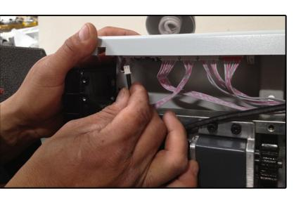
3. Lift up on the top cover and remove the black cable connected to the pc board.
