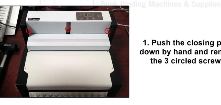
1. Push the closing plate down by hand and remove the 3 circled screws.
