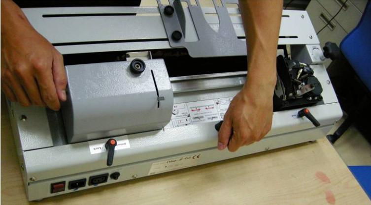
2. Loosen the both side screws at back side.
