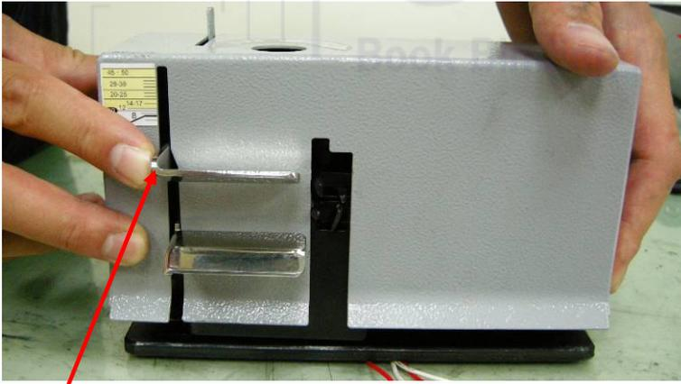
Tip: To remove the cover easily, Finger push the coil hold device
