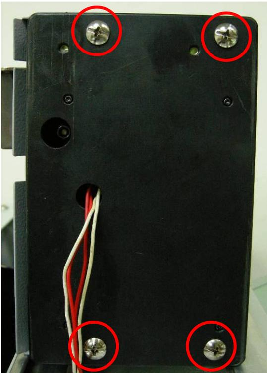
10. Remove the Cover of Crimping Unit.
