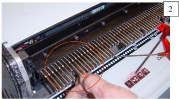
3A) Use a 4mm allen wrench to loosen die-disengagement mechanism. Two bots on left and two bolts on right must be removed.
