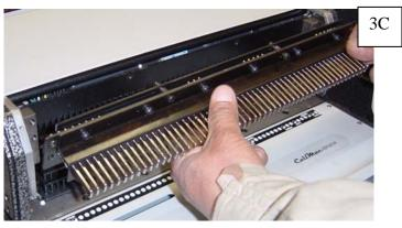
4) **Remove old or damage die.** Use pliers to grab and pull die up. Hint: Use opposite hand to hold pin after each upward pull and gradually remove it. See pictures 4A, 4B and 4C
