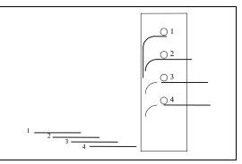
\* Note: For the right paper ejection, the same setting can be performed by the d value. The paper stacked on the first-station shelf comes out first but is ejected to the bottom of an ejected collation set on crisscross stacker.
