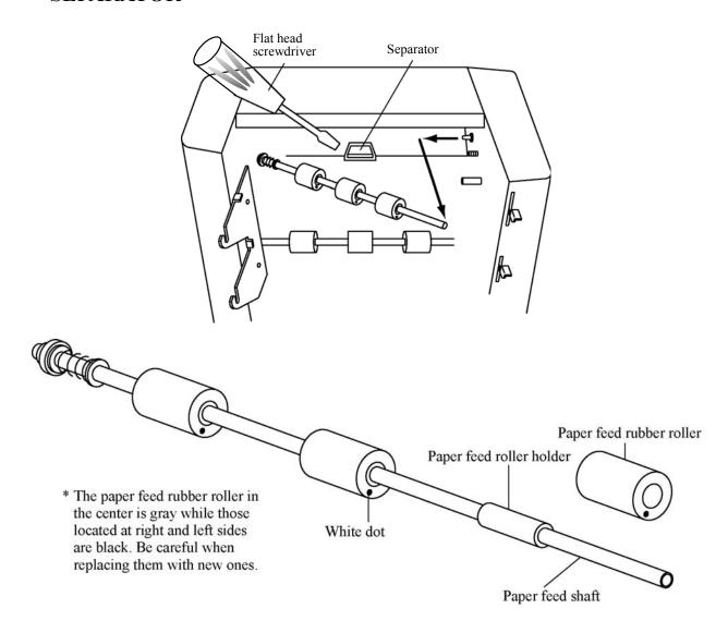
• Replacement of paper feed rubber rollers
