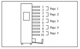
• Loading paper with the printed side down in Alternate mode
