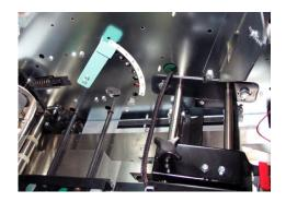
Under extreme circumstances, when the cover sheet tends to be torn from the rest of the set, this can be rectified by adjusting the Fold Adjust Levers located above the pre-fold transport. There are eight positions for each lever. The topmost notch is the default position. Move the lever notch by notch until performance is satisfactory.
